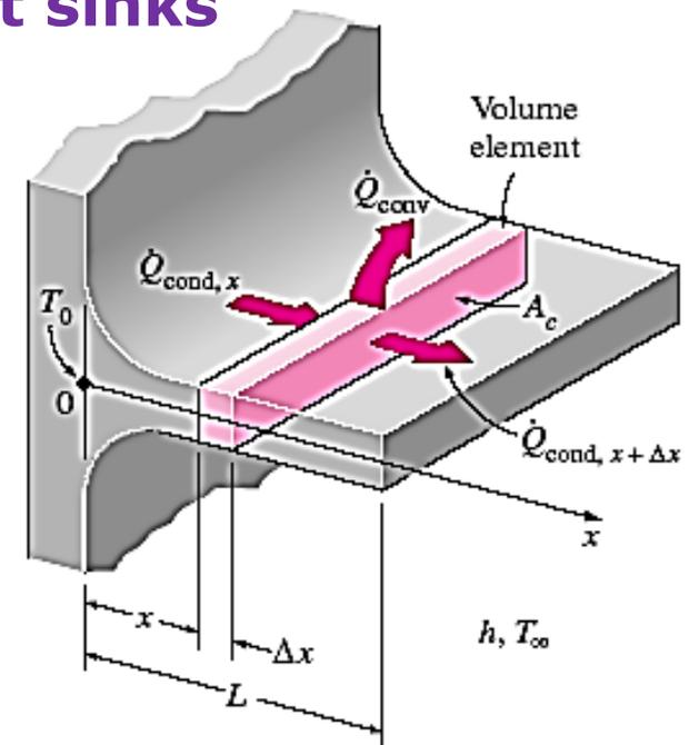
Volume element of a fin at location  $x$  having a length of  $\Delta x$ , cross-sectional area of  $A_c$ , and perimeter of  $p$ .
