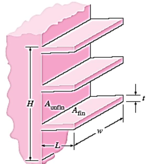
$$\begin{aligned}A_{\text{no fin}} &= w \times H \\ A_{\text{unfin}} &= w \times H - 3 \times (t \times w) \\ A_{\text{fin}} &= 2 \times L \times w + t \times w \text{ (one fin)} \\ &= 2 \times L \times w\end{aligned}$$
