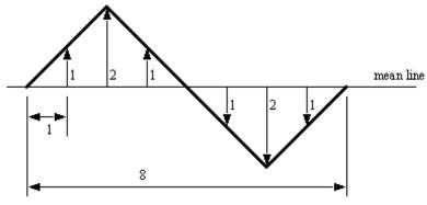
We can find the surface roughness using heights,
