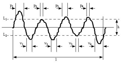
The two parallel lines  $L_1$  and  $L_2$  are positioned such that the y cut off the peaks and valleys, given the mathematical constraints,
