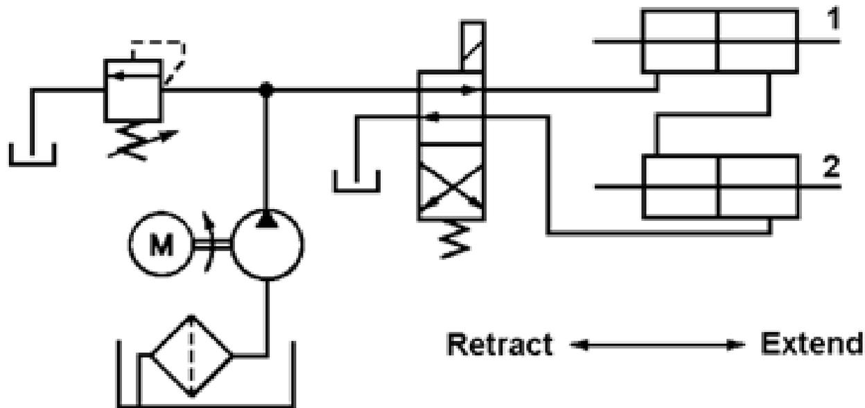
**Synchronous circuit using equal area cylinders**
