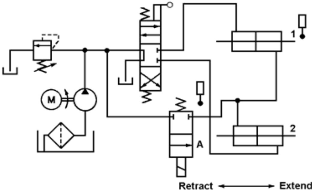
Replenishing synchronous circuit
