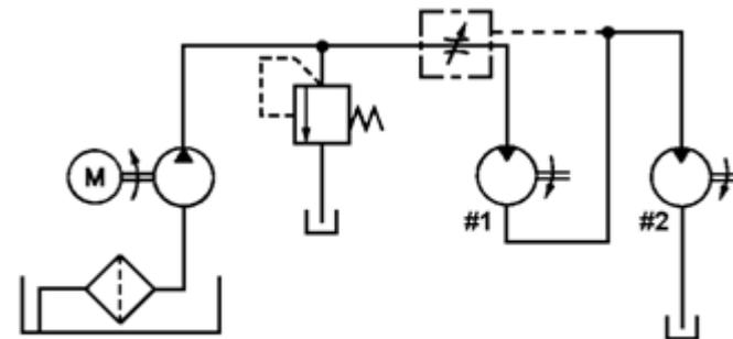
C-Q conveyor circuit with flow control valve
