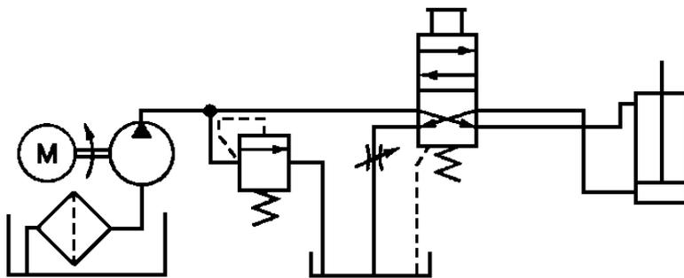
C-Q circuit; meter-out control
