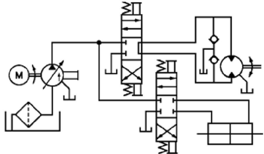
*C-P circuit with two actuators*
