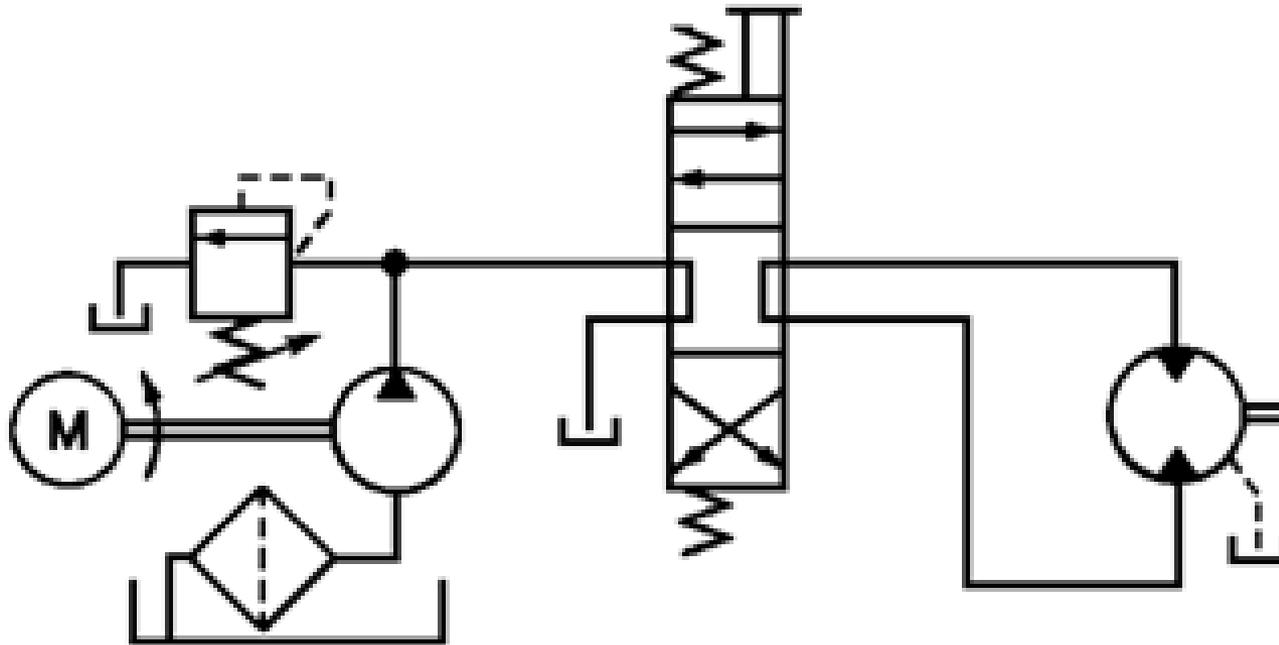
**Open-center circuit with rotary actuator**
