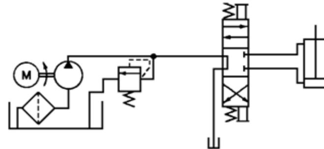
C-Q circuit with open-center control valve and pilot operated relief valve
