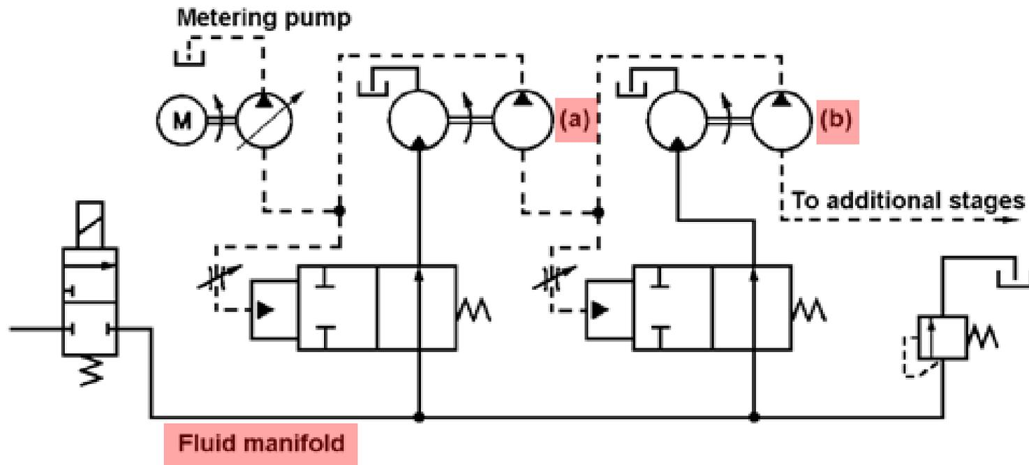
**Conveyor fluid motor control circuit**
