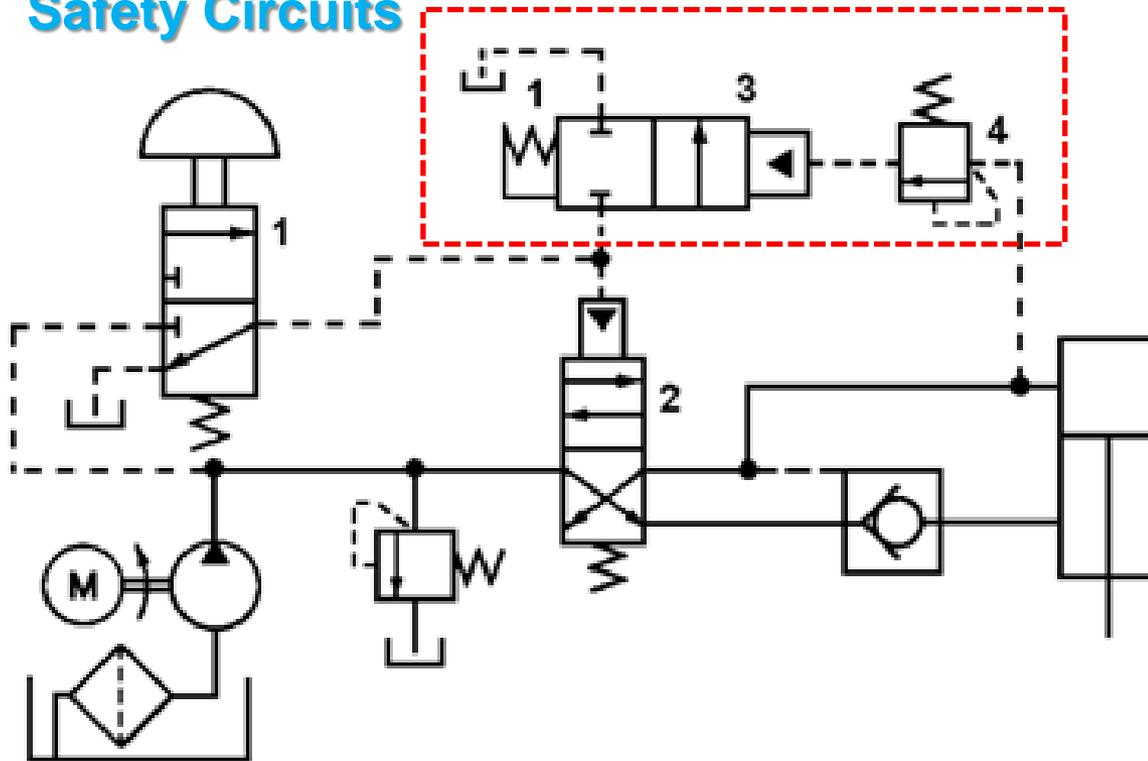
Operating the three-way manual control valve will have no effect on the circuit unless detented overload valve 3 is reset manually.
