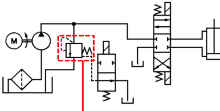
Pilot relief valve controlled by solenoid
