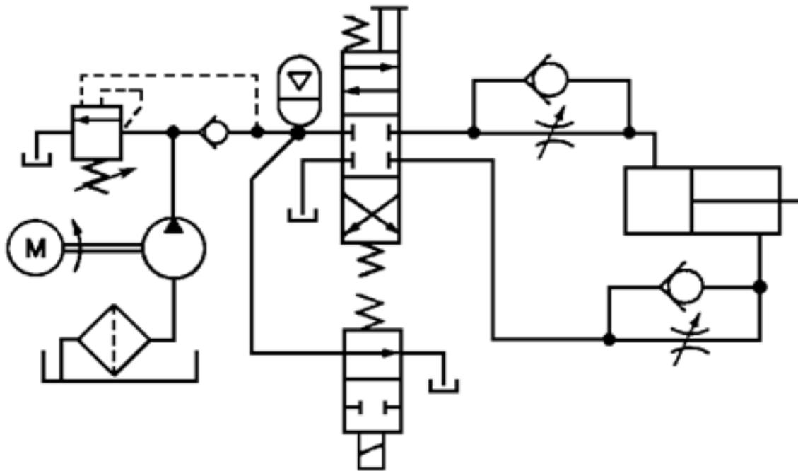
Closed-center accumulator circuit
