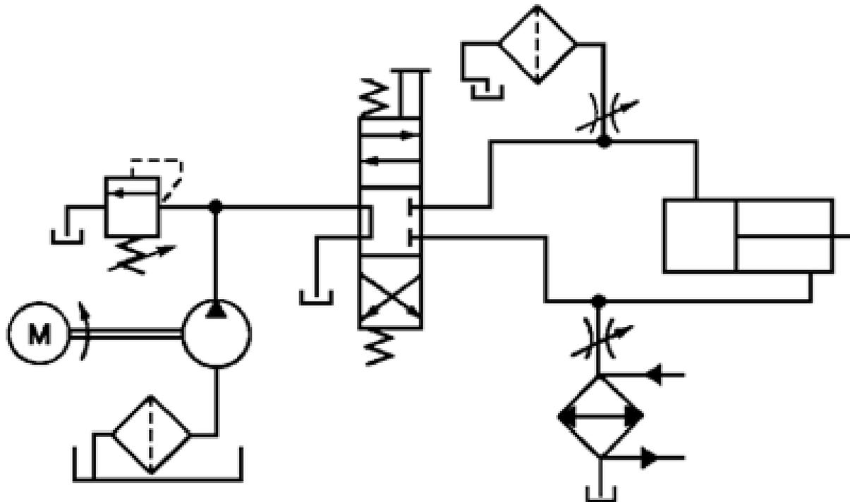
**Open-center bleed-off circuit with filter and heat exchanger**
