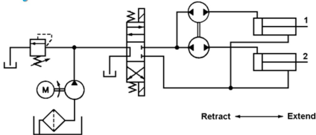
Synchronous circuit using flow divider
