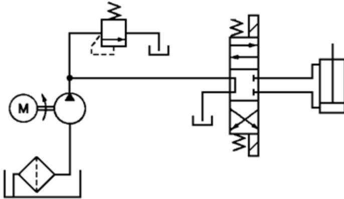
Open-center circuit with linear actuator
