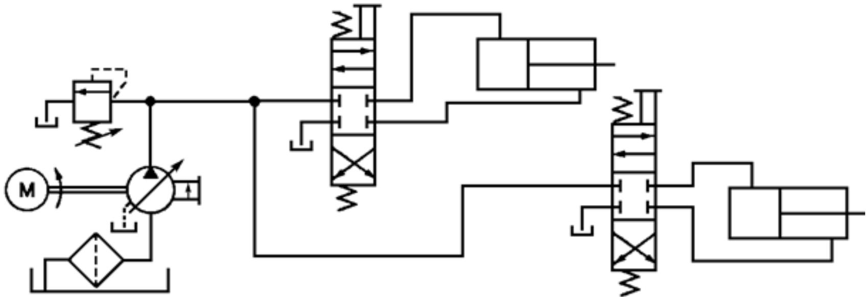
**Closed-center circuit with variable displacement pressure compensated pump**
