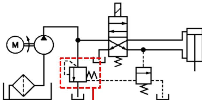
Pilot relief valve controlled by pilot valve
