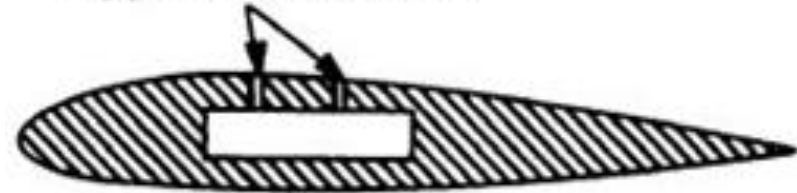
Boundary layer control by upper surface suction
