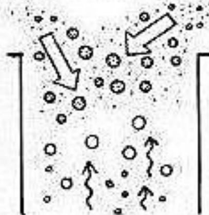
A "flue" mix of lime or limestone and water is sprayed into the sulfur dioxide gas in the scrubbers.
