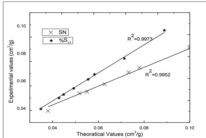
**Fig. 2** Theoretical and experimental total mass attenuation coefficients for S<sub>17</sub> and S<sub>N</sub> alloys
