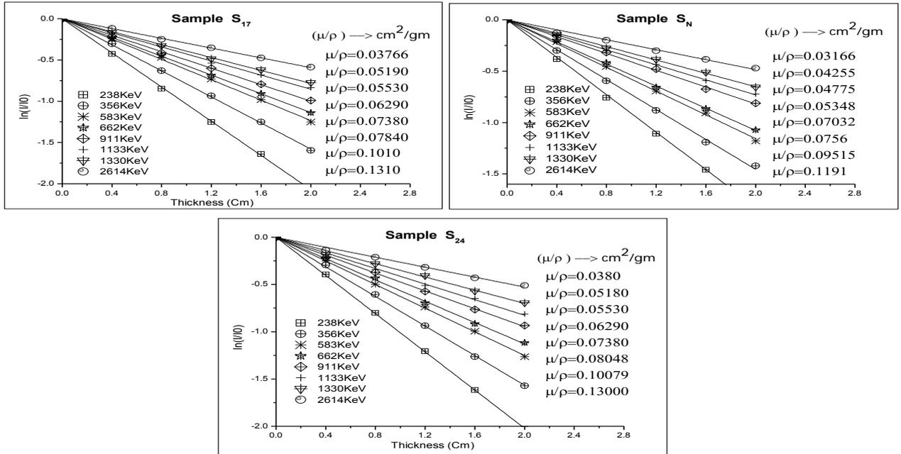
**Fig. 1** Mass attenuation coefficients for the steel alloys at different energies.
