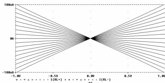
**Fig. 4: DC Transfer Characteristics of The Proposed DCBOTA**
