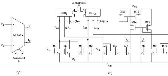
Fig. 1: Proposed DCBOTA (a) Symbol (b) CMOS Realization
