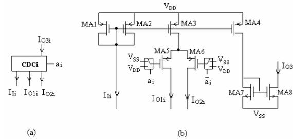
Fig. 3: Proposed CDC (a) Symbol (b) CMOS Realization
