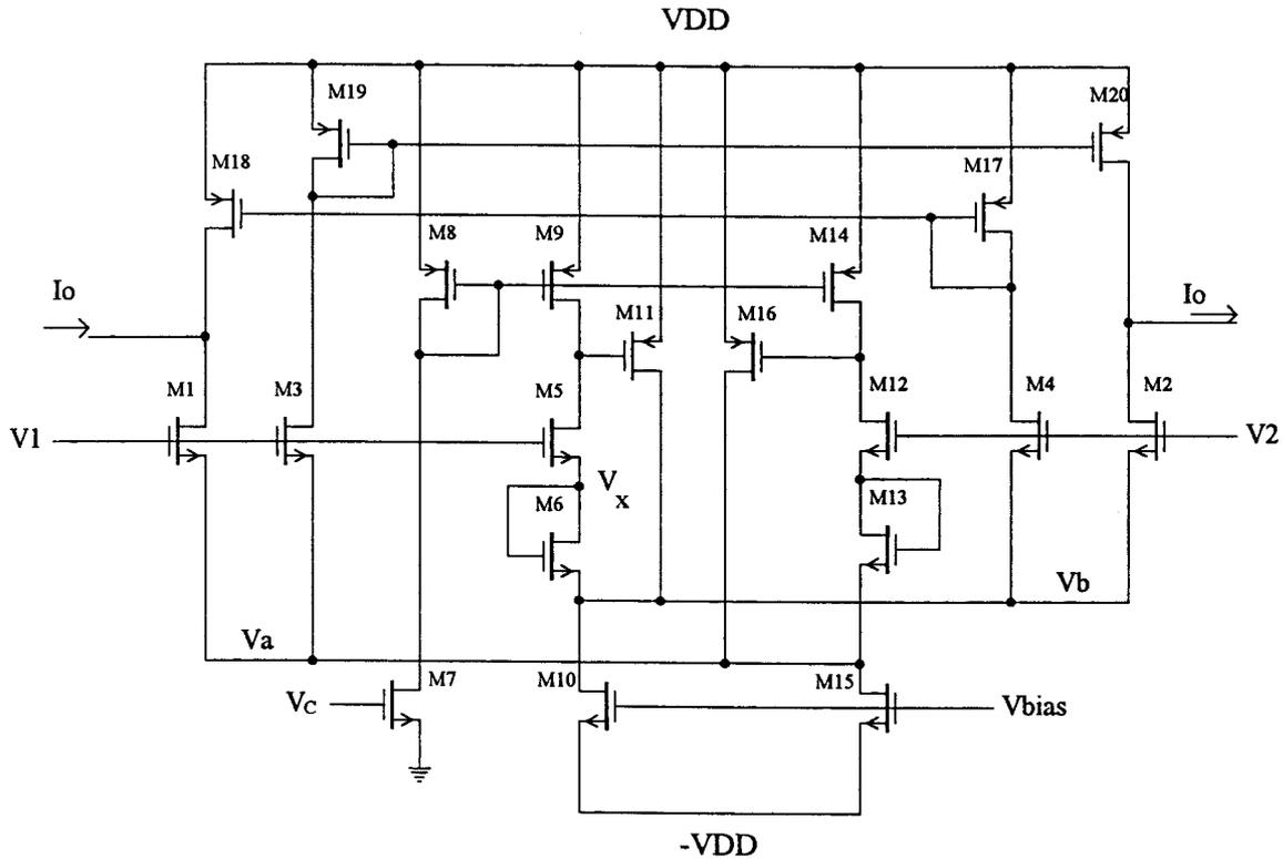
Fig. 2. The CMOS circuit of the BOTA.
