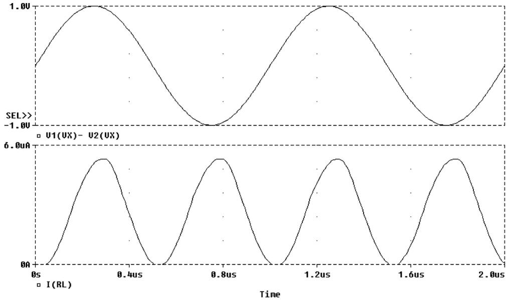
Fig. 13. The voltage-mode multiplier as a frequency doubler.
