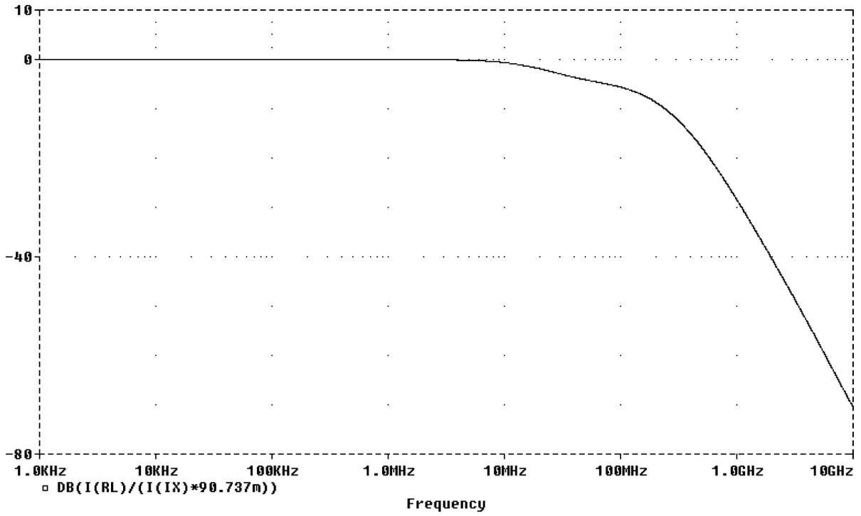
Fig. 7. Normalized frequency characteristics of the proposed current-mode multiplier.
