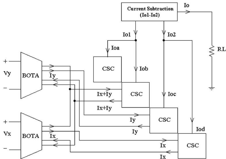
Fig. 4. Block diagram of the proposed voltage-mode multiplier.
