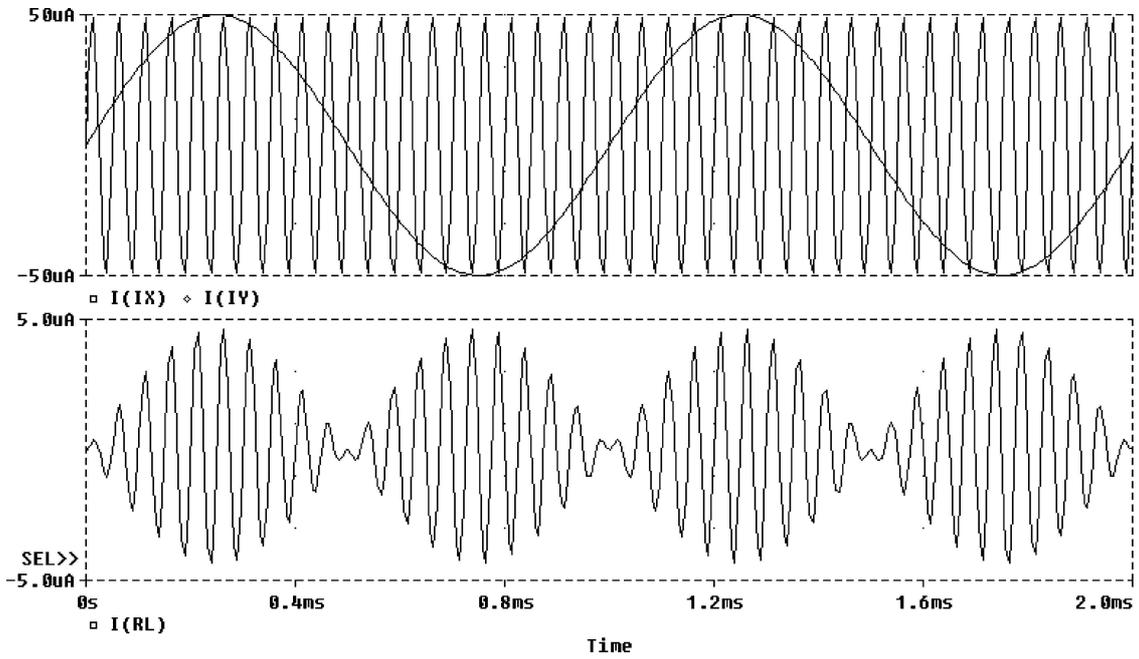
Fig. 8. The current-mode multiplier as an analog amplitude modulator.
