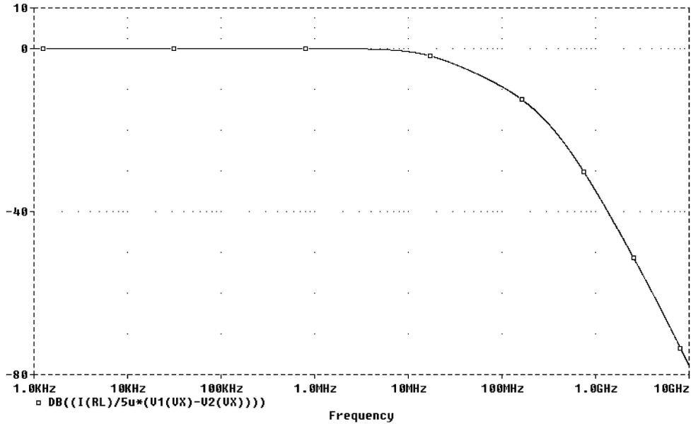
Fig. 11. Normalized frequency characteristics of the proposed voltage-mode multiplier.
