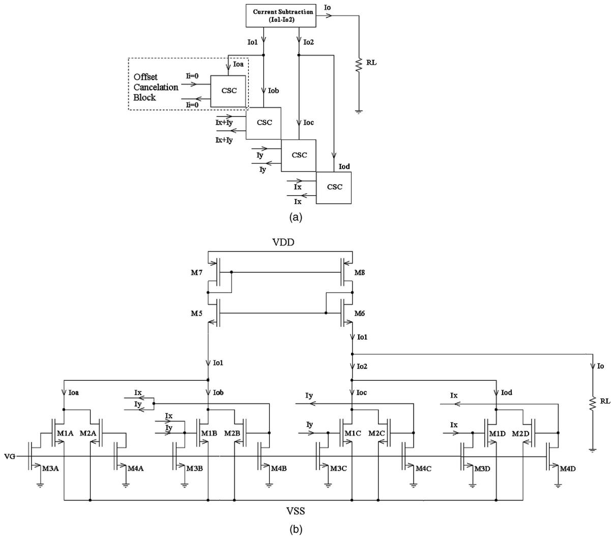
Fig. 2. (a): Block diagram of the proposed current-mode multiplier, (b): CMOS realization of the proposed current-mode multiplier.
