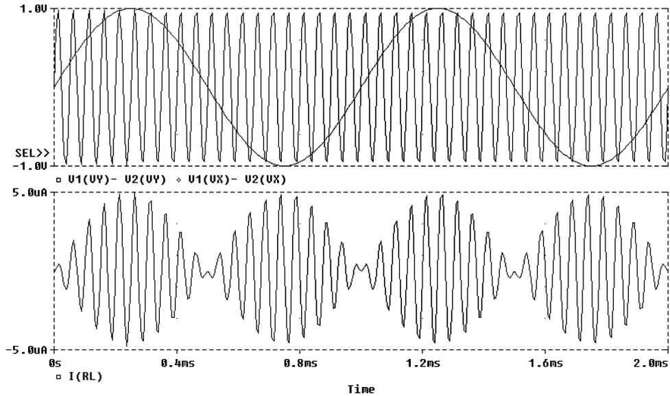
Fig. 12. The voltage-mode multiplier as an analog amplitude modulator.
