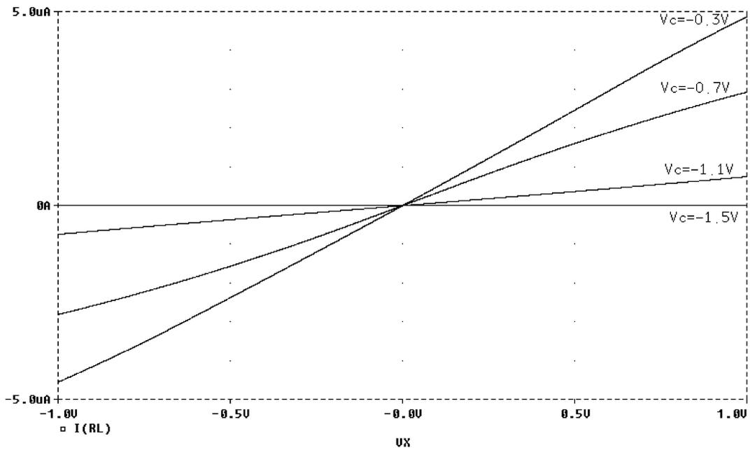
Fig. 14. DC transfer characteristics of the proposed voltage-mode multiplier with  $V_C$  as a parameter and  $V_Y = 1$  V.
