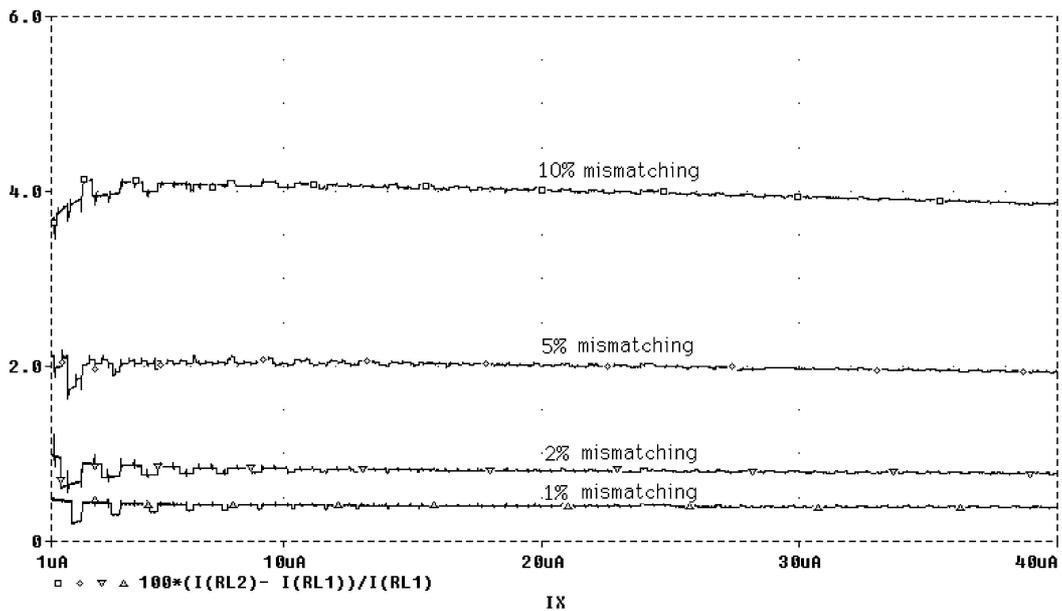
Fig. 6. Percentage error of the output current of the current-mode multiplier due to mismatching effect (at 1, 2, 5 and 10% of mismatching).
