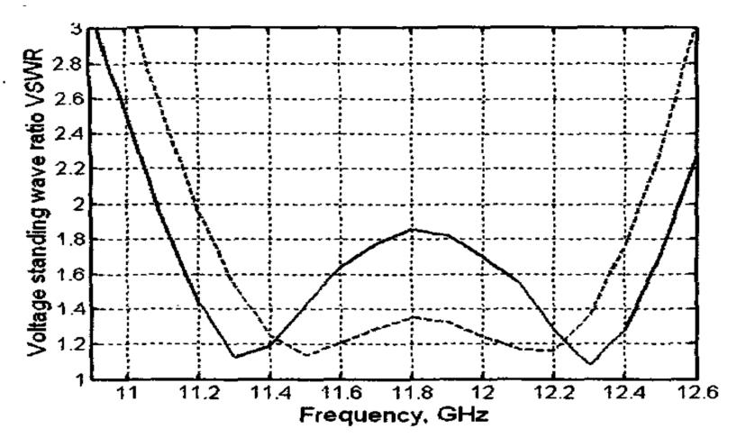
The VSWR of the aperture-coupled microstrip antenna without matching (solid line) and with matching (dashed line).
