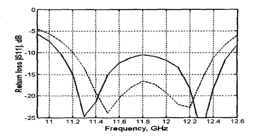
The return loss of an aperture-coupled microstrip antenna without matching (solid line) and with matching (dashed line)
