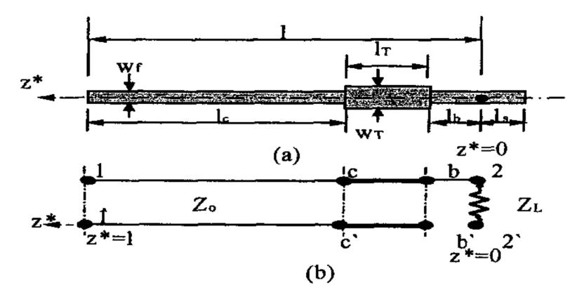
The microstrip feed line and its equivalent circuit. Normal TL analysis follows, the quarter-wavelength transformer must be placed a distance  $l_b$  away from the load at point  $z^*=0$ , where the input impedance toward the load at  $z^*=l_b$  is real. The distance  $l_b$  can be found from Equation  $x(l_b)=0$
