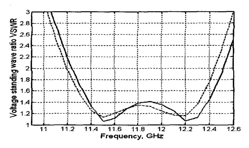
A comparison of the aperture-coupled microstrip antenna's bandwidth with the proposed matching for simulated (dashed line) and measured (solid line) antennas.
