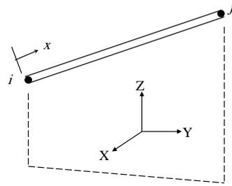
Figure 3. The geometry, node locations and coordinate system of Link8 element
