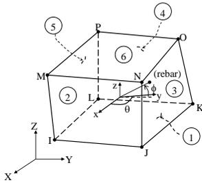
Figure 2. The geometry, node locations and coordinate system of Solid65 element
