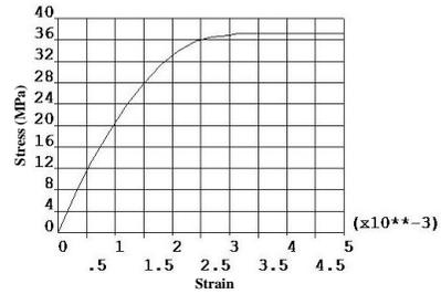
Figure 7. Stress-strain curve for utilized concrete ( $f'_c = 37.2$  MPa)
