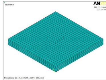
Figure 5. Meshed elements (solid65) for modeling concrete and cementitious slabs
