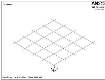
Figure 4. Meshed elements (link8) for modeling reinforcement grid
