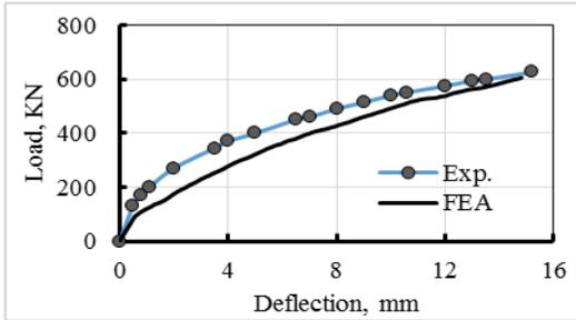
Figure 14. Load-Deflection response, LD slab
