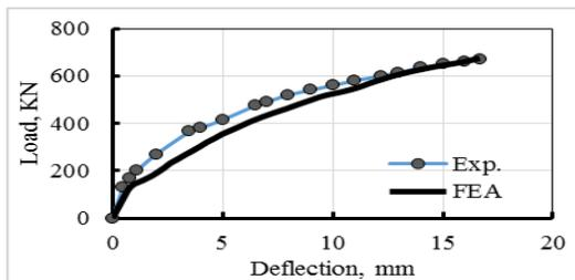
Figure 12. Load-Deflection response, NN slab
