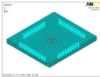
Figure 8. Restraints and applied displacements for first group
