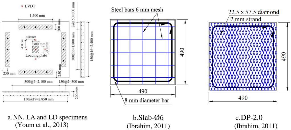
Figure 1. Specimen dimensions and steel reinforcement details.
