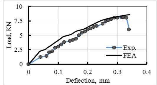
Figure 15. Load-Deflection response, Slab-I
