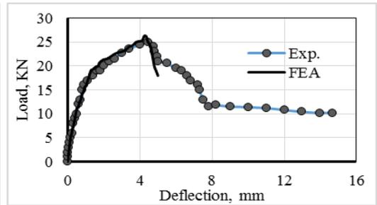
Figure 17. Load-Deflection response, DP-2.0 slab
