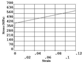
Figure 6. Stress-strain curve for steel bars 10 mm
