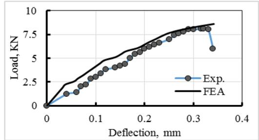
Figure 15. Load-Deflection response, Slab-I
