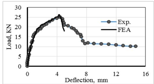
Figure 17. Load-Deflection response, DP-2.0 slab
