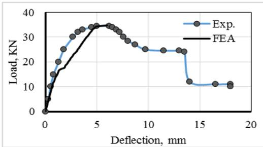
Figure 16. Load-Deflection response, Slab-Ø6
