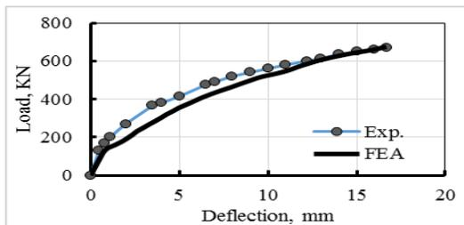
Figure 12. Load-Deflection response, NN slab
