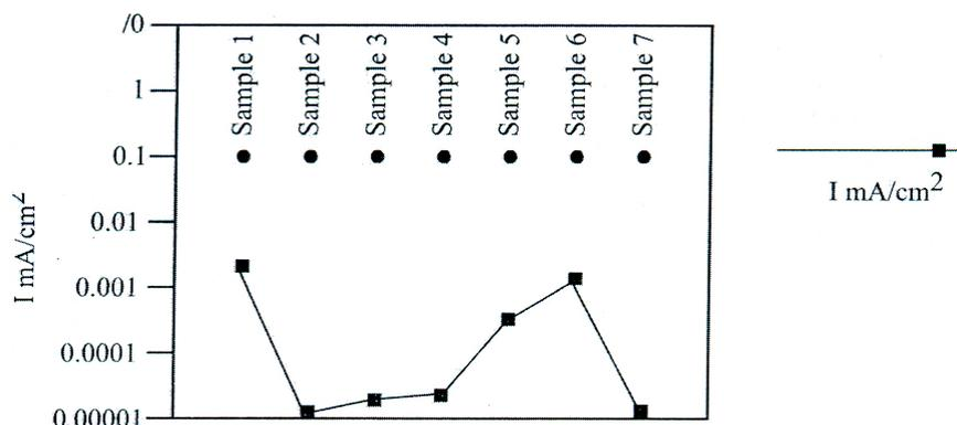
**Fig.7- Declares the change in the density of corrosion current of the tested samples.**
