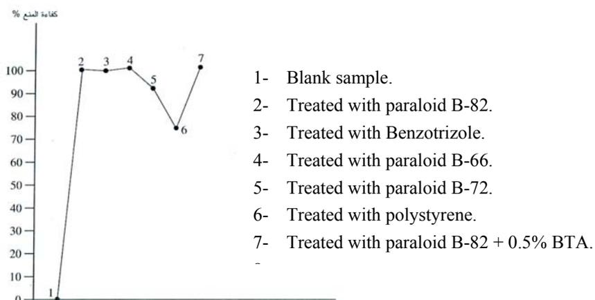
**Fig.8- shows the efficiency of the applied Inhibitors through electrochemical measurements (polarization test).**
