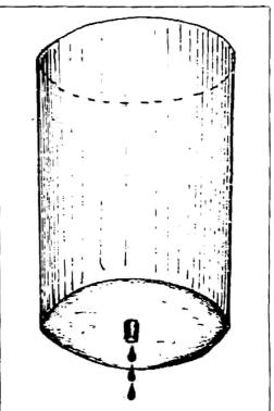
Fig. 1. Metal cylinders 32 cm. in diameter, 80 cm. in depth and terminating in a hole 2 cm. diameter.
