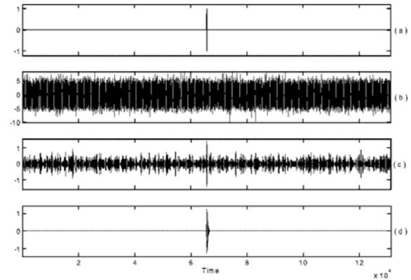
**Figure 7.** (a) Clean signal (b) Noisy signal SNR = -20 dB (c) denoised signal after the first stage (d) denoised signal after the second stage (step 5)
