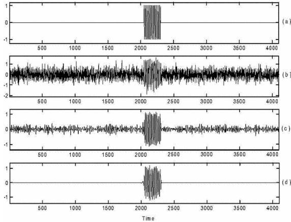
**Figure 6.** (a) The clean RF radar pulse  $z(n)$  (b) The received noisy RF radar pulse  $x(n)$ , SNR = -3 dB (c) The result of the first stage (d) The result of the second stage (step 5).
