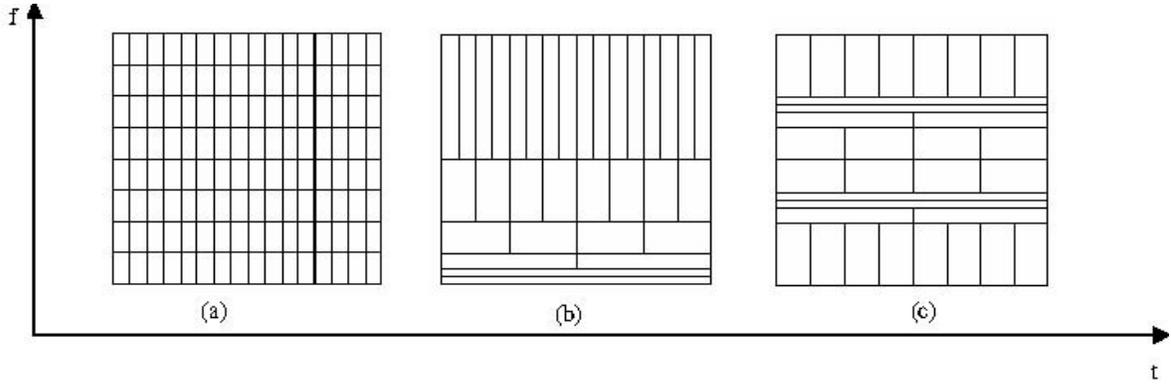
**Figure 1.** Tiling the time-frequency plane (a) Windowed Fourier transform (b) Wavelet transform (c) Wavelet packet transform
