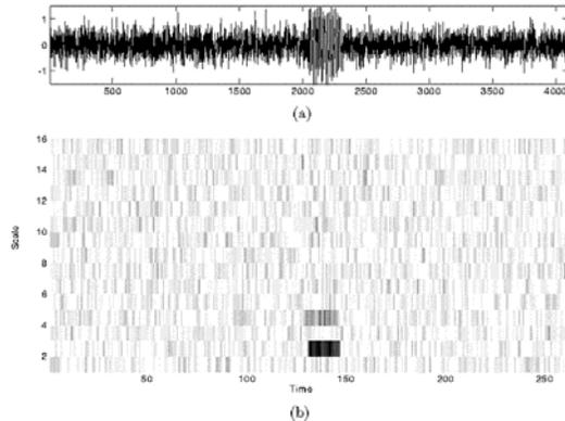
**Figure 4.** (a) The received noisy radar pulse  $x(n)$ , SNR =  $-3$  dB. (b) The wavelet packet coefficients of  $x(n)$ ,  $J = 4$ .
