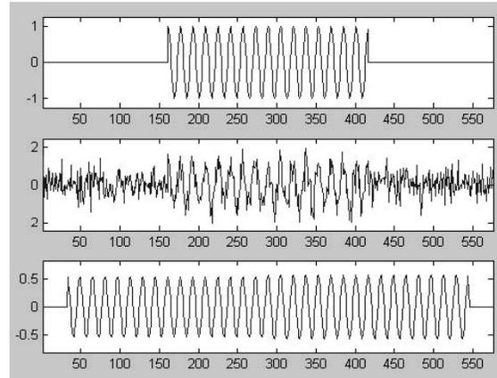
**Figure 10.** Result for signal denoising using windowed Fourier transform.
