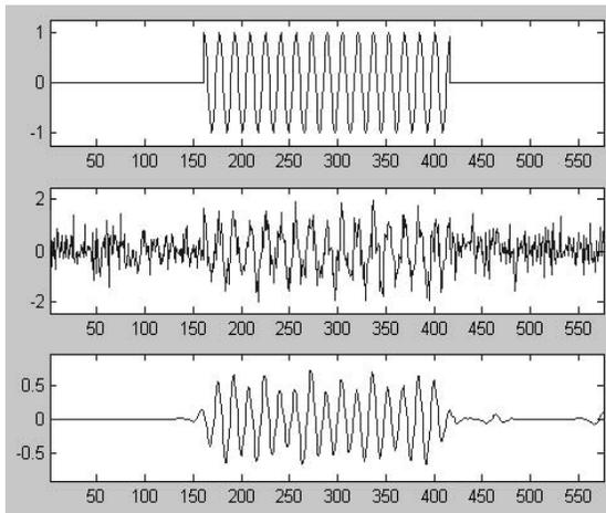
**Figure 9.** Result for signal denoising using wavelet packet Transform.
