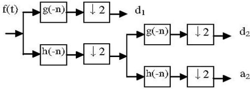
**Figure 2.** Filter bank implementation of discrete wavelet decomposition.
