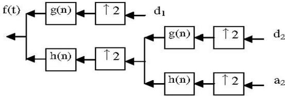
**Figure 3.** Filter bank implementation of discrete wavelet reconstruction.
