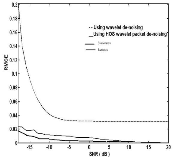
**Figure 8.** RMSE as a function in SNR for the proposed technique and the wavelet denoising in MATLAB.
