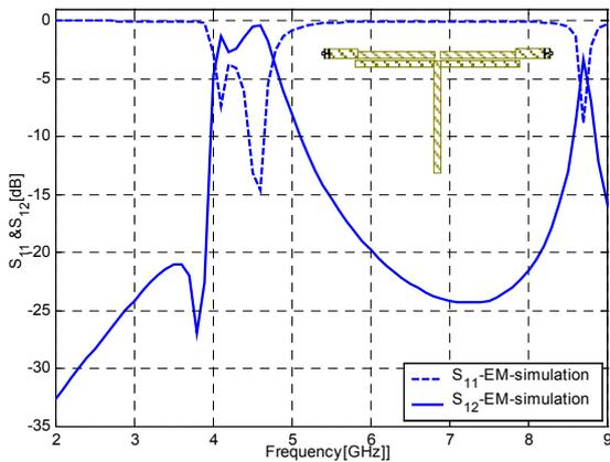
Fig. 4., 5.  $S_{11}$  &  $S_{12}$  of Structure 1. & Structure 2
