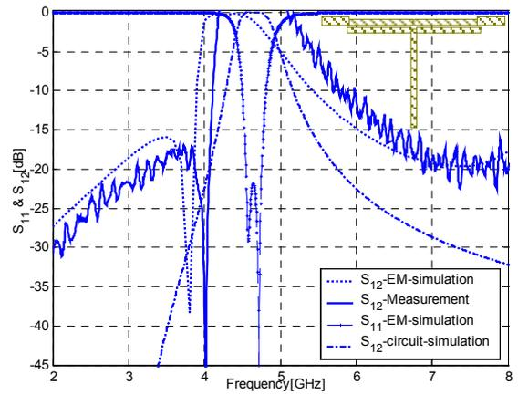
Fig. 6 The comparison of  $S_{12}$ -Parameters
