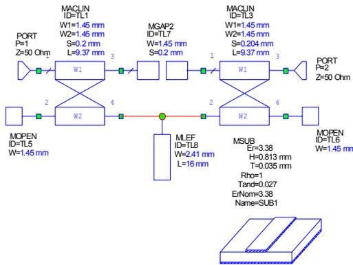
Fig. 8 Equivalent circuit network of the proposed BPF
