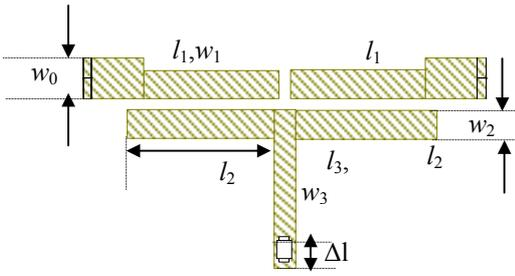
Fig.3 BPF with short- circuit (Structure1),  $l_1=l_2=9.37mm, l_3=5.37mm, w_1=1.45mm, w_2=1.25mm, w_3=1.85mm$
