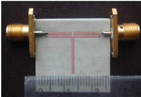
Fig. 9 Photograph of fabricated BPF (Structure3)
