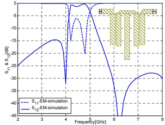
Fig. 7 The response  $S_{12}$  of Structure 3
