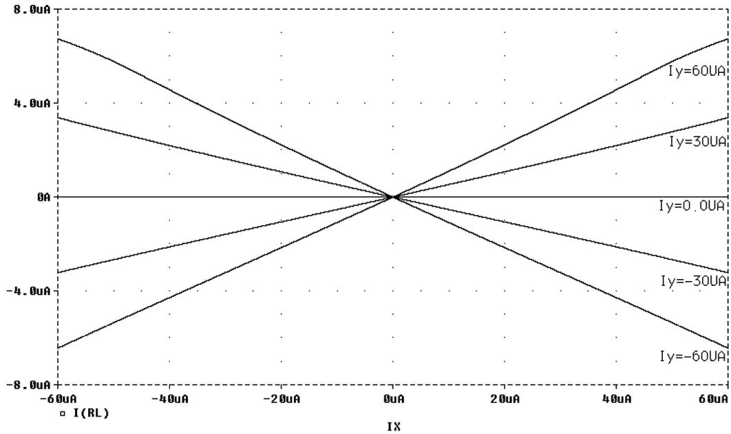
Fig. 5. DC transfer characteristics of the proposed current-mode multiplier of Fig. 2.
