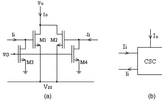
Fig. 1. (a): CMOS realization of the proposed squarer cell, (b): Symbol of the proposed squarer cell.
