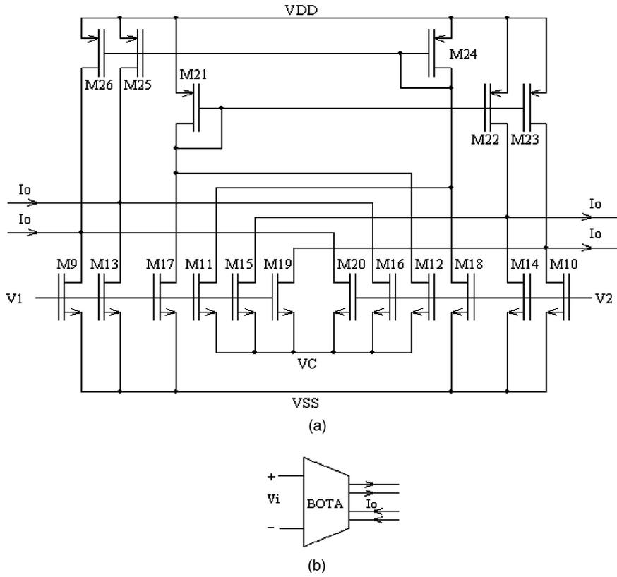
Fig. 3. (a): CMOS realization of the balanced output transconductor (BOTA) [1], (b): Symbol of the balanced output transconductor (BOTA) [1].
