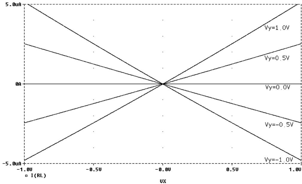
Fig. 10. DC transfer characteristic of the proposed voltage-mode multiplier of Fig. 4.
