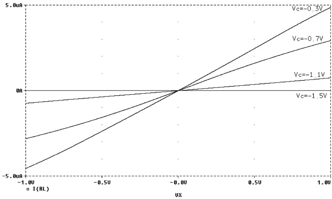
Fig. 14. DC transfer characteristics of the proposed voltage-mode multiplier with  $V_C$  as a parameter and  $V_Y = 1\text{ V}$ .
