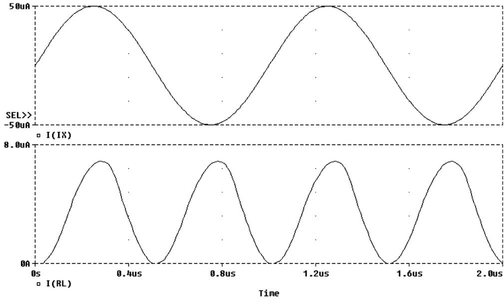
Fig. 9. The current-mode multiplier as a frequency doubler.
