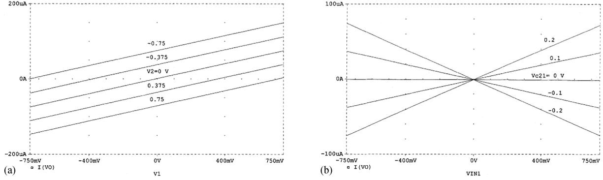
Fig. 5. (a) The output current of the transconductor cell, (b) the output current of the multiplier cell.
