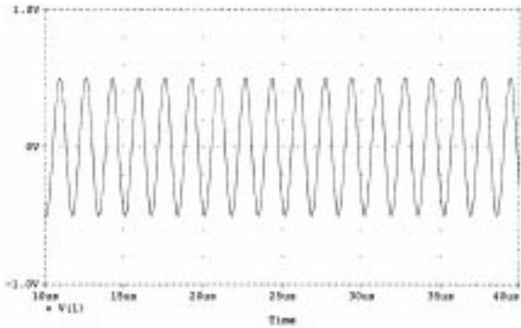
Fig. 11(c). The voltage waveform  $V_1$  of the oscillator using ideal CFOA.
