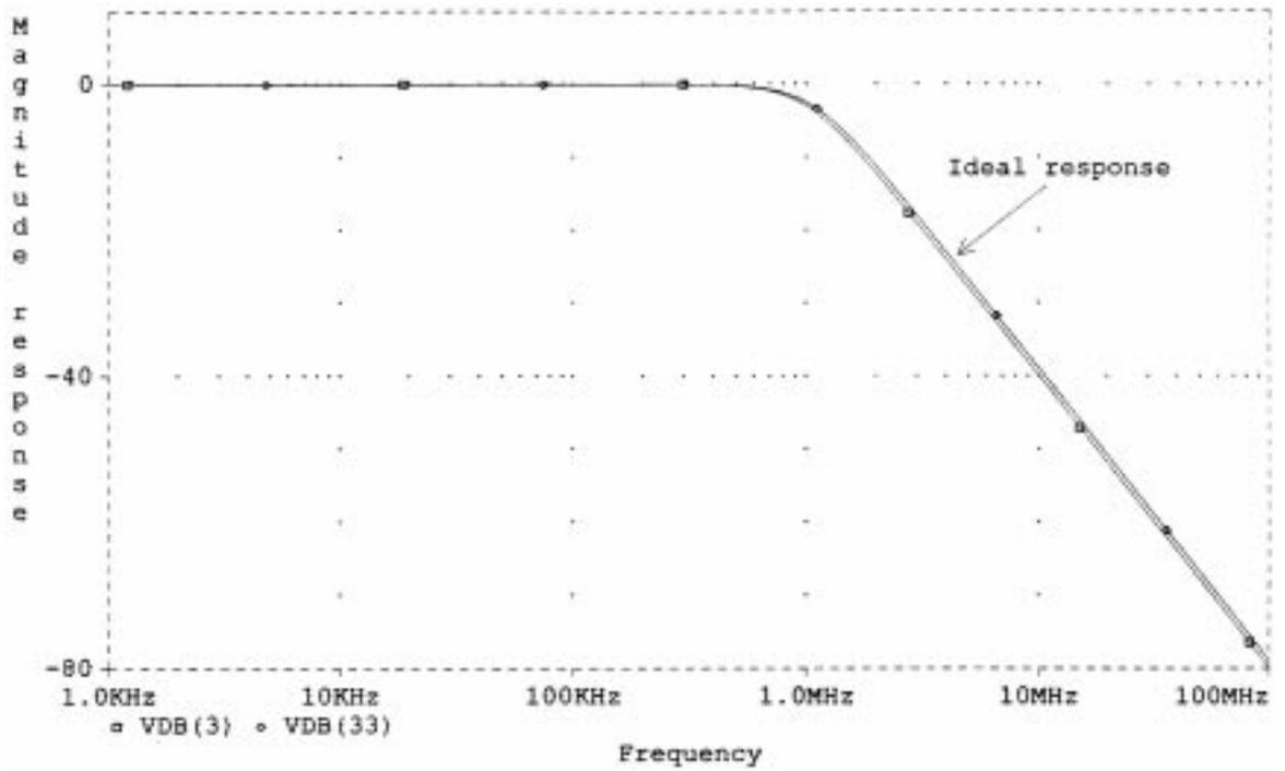
Fig. 9(c). The magnitude response of the lowpass filter.
