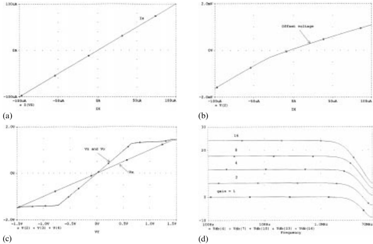
Fig. 3. (a) The Z terminal current, (b) the X terminal offset voltage, (c) the voltage swing at the X, Z, and the O terminals of the CFOA based amplifier, (d) the frequency response of the CFOA based amplifier for different values of gain.
