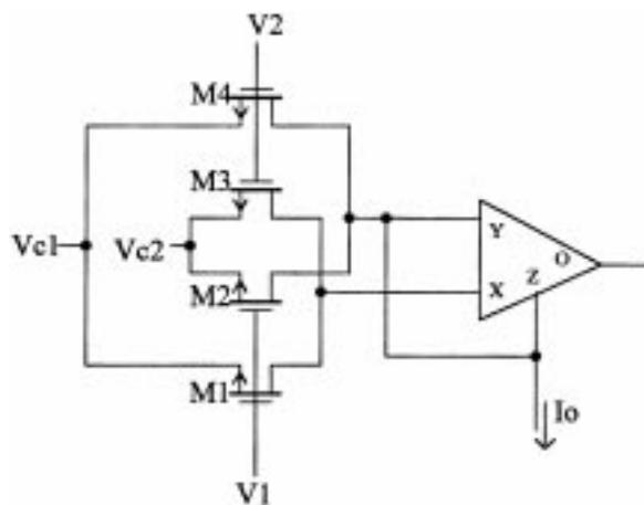
Fig. 4. The transconductor/multiplier cell.
