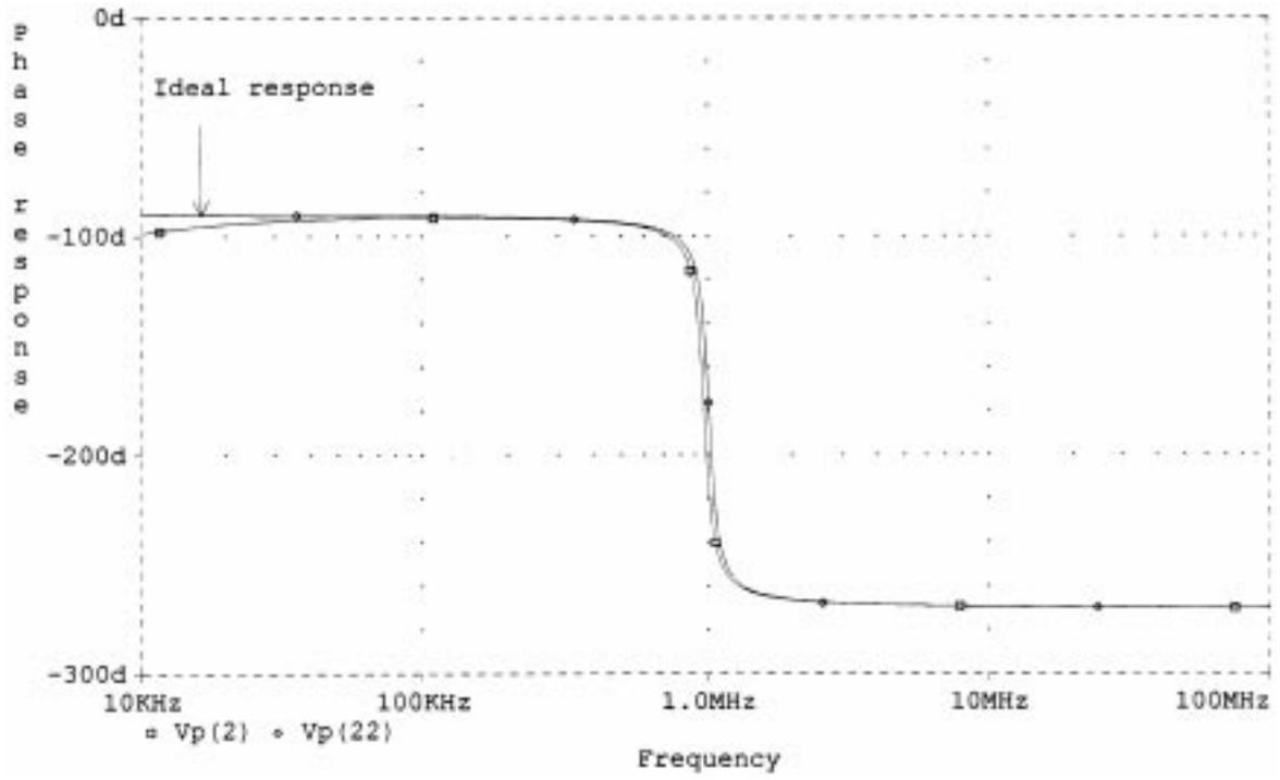
Fig. 9(b). The phase response of the bandpass filter.
