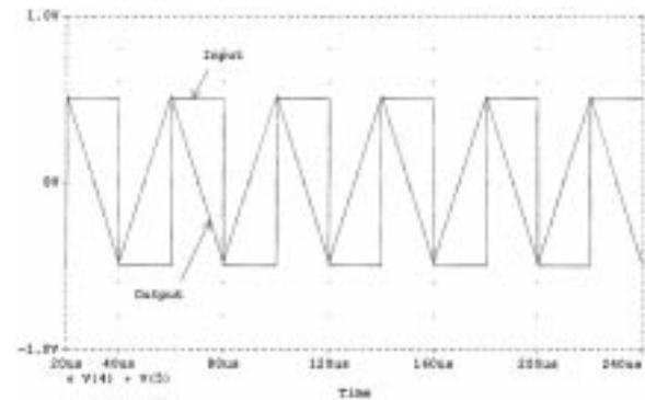
Fig. 7. The output of the integrator along with the square wave input signal.
