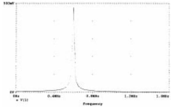
Fig. 11(d). The frequency spectrum of the oscillator using ideal CFOA.
