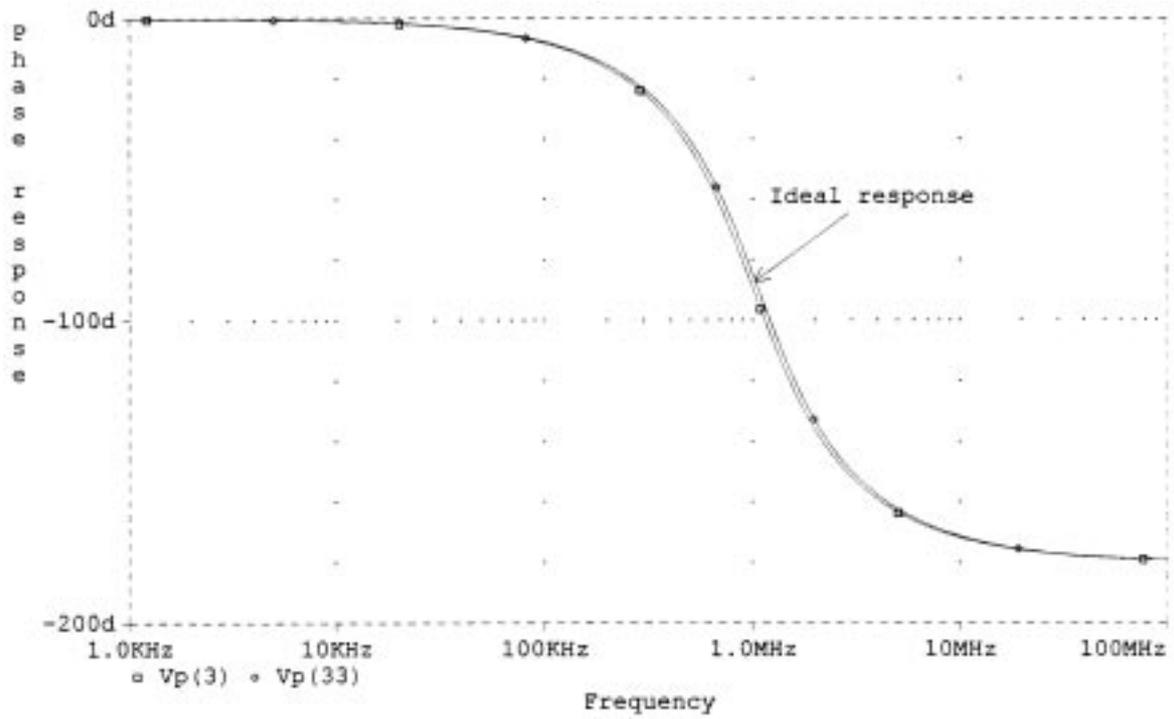
Fig. 9(d). The phase response of the lowpass filter.
