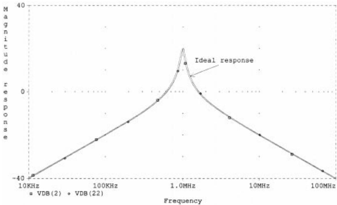
Fig. 9(a). The magnitude response of the bandpass filter.
