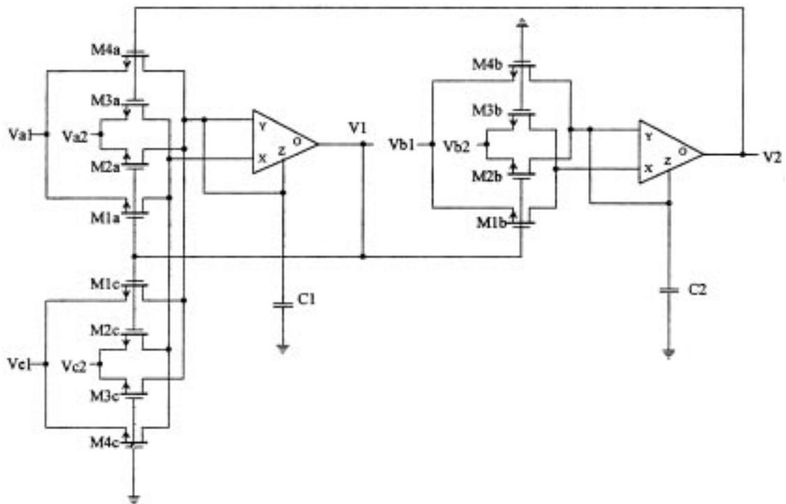
Fig. 10. The MOS-C CFOA oscillator.
