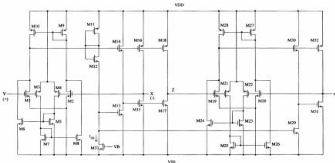
Fig. 2. The rail to rail CFOA CMOS circuit.
