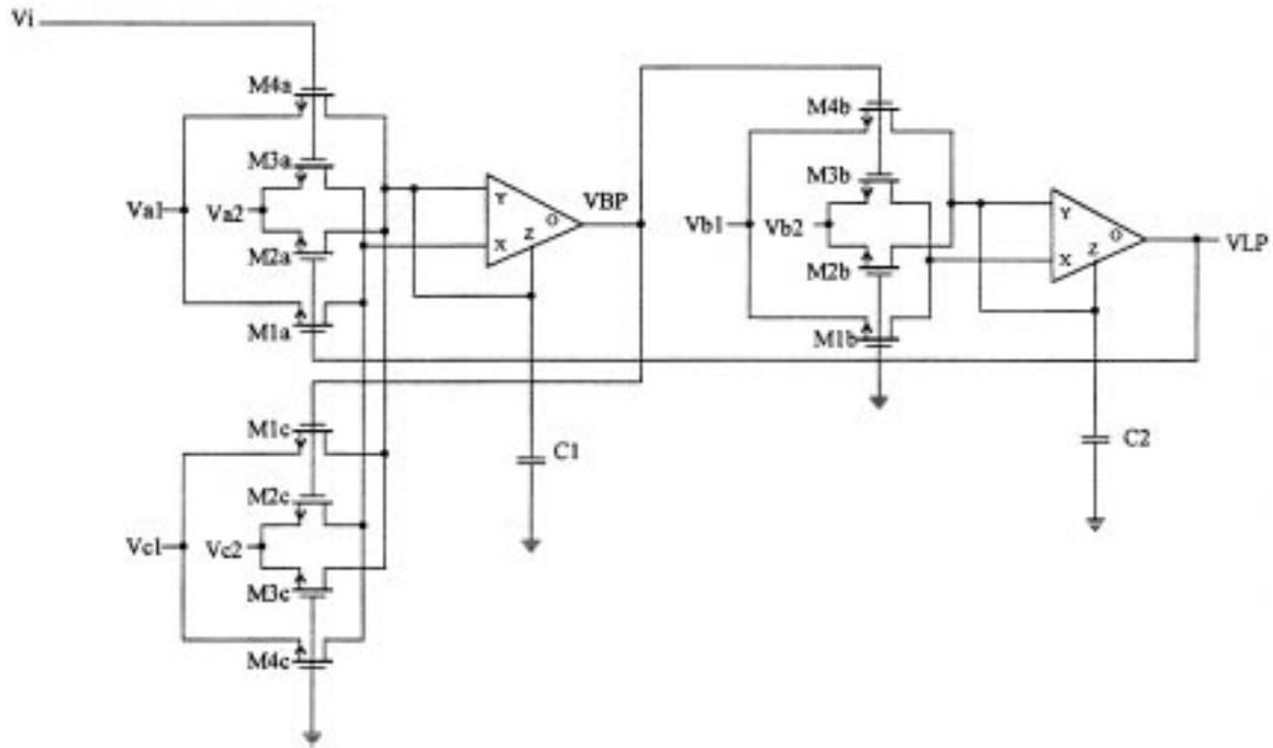
Fig. 8. The CFOA bandpass-lowpass filter.
