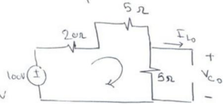
at  $t \geq 0$  switch closed
