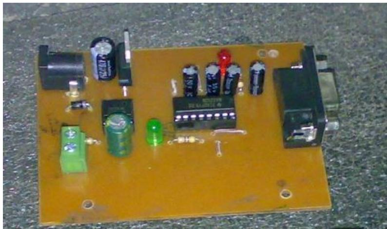
Figure 30 RS232 to 485 Converter Top view
