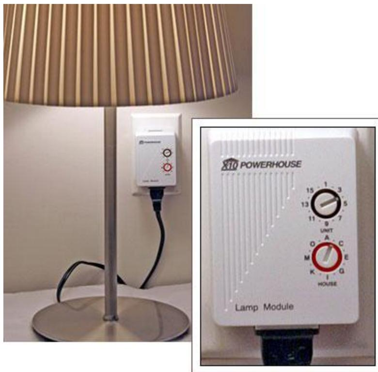
Figure 108 An X10 lamp module turns a lamp on and off when an X10 signal is sent from an X10 transmitter
