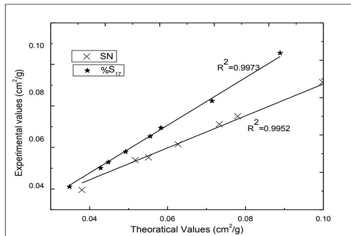
**Fig. 2** Theoretical and experimental total mass attenuation coefficients for  $S_{17}$  and  $S_N$  alloys
