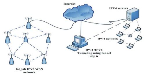
Fig. 4: Contiki Tunslip6 process, a tool used to bridge the wireless IPv6 network traffic onto a PC connected to IPV4 network (ipv4/ipv6 tunneling).
