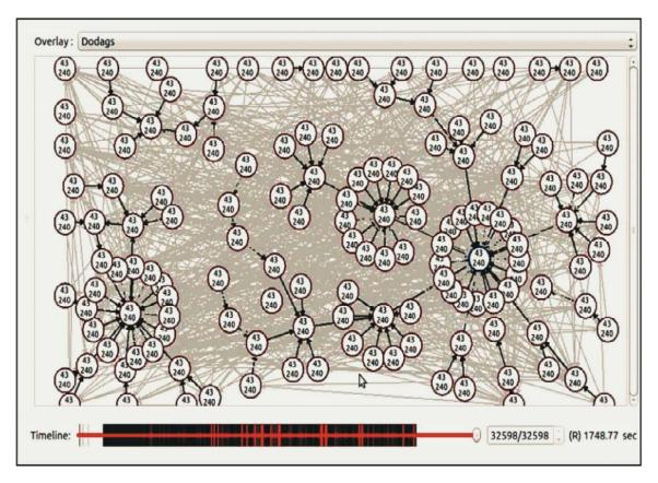
Fig. 5: The experimental multi-hop logical topology. Snapshot of foren6 GUI for the RPL operation during the experiment when all nodes joined the DODAG and form their routing tables
