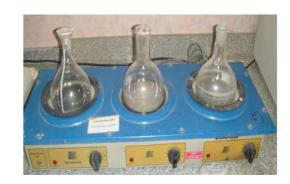
A system for heating samples.
