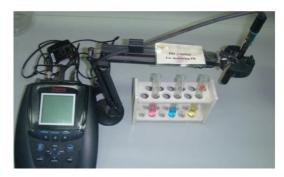
A system for measuring PH or concentration and Temp. of the sample with automatic blank correction selection.
