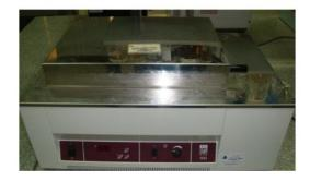
Shaking device operates with a temperature range between approximately 5°C above ambient temperature to 99.9°C, the shaking frequency can be set in a range of 10- 250 / min
