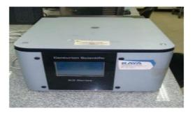
A system for centrifuging samples with a maximum speed 6000 rpm
