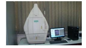
A system for running a wide variety of protocols including nucleic acid gels, protein gels, complete analysis of bands and plots.
