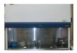
working under normal laboratory condition. do not use any aggressive media for cleaning the surface
