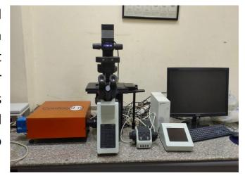
Type laser confocal microscope: Confocal laser scanning microscopy (CLSM) allows optical slicing through tissue. By eliminating out-of-focus images: CLSM affords greater spatial resolution in living tissue and allows visualization of living structure as small as dendritic spines.
