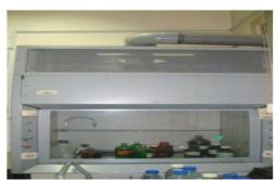
Air clean system designed to protect the operator , the process , or both from toxic vapors , fumes , gases and particles . so , it is a system for operation with specific toxic and mutagenic chemicals .
