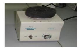
**A** system for mixing samples in small tubes or eppendorf tubes.
