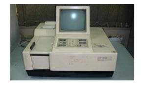
A system for measuring DNA concentration and its contamination with RNA or protein (automatic determination of concentration)
