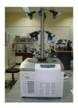
It is the most gentle process for drying products (extraction of water from frozen material), based on sublimation which meaning direct conversion from solid to gaseous state avoiding the liquid state, this happen under vacuum (pressure lower than 6.11 m bar) and the temperature in the product is less than -10°C
