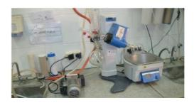
It is a device used for gentle removal of solvents from samples by evaporation (under reduced pressure).
