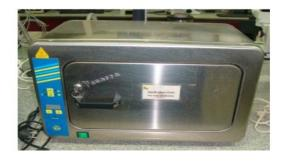
The system operates under Temp. between 140 and 250 °C, time can be set between 1 min and 600 min. the cycle is considered valid only if the writing END is appearing.
