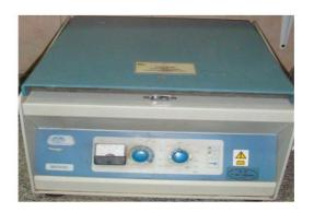
A system for centrifuging samples with a maximum speed in RPM : 8000 u / min.
