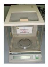
Weight very small solid samples (capacity 220.0000 gm). It takes about 6 seconds to display a stable and accurate weigh difference between sample temp. and that of the weighing chamber may take several minutes to equilibrate, weighing errors may be greater than 1mg whet the temp. in the lab. Changes TARE key clears the display to zero.
