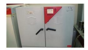
A system for stimulating the parameters of natural conditions as temp., humidity and light or any climatic conditions for a long period of time constantly.
