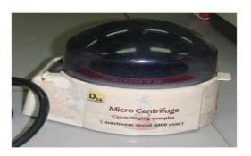
A system for centrifuging samples with a maximum speed 6000 rpm
