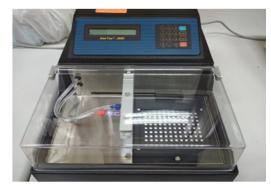
Microplate washers are laboratory instruments designed to control the procedure of washing experimental samples arranged in plate-based formats. Users load a plate and select a program; microplate washers then dispense, soak and aspirate liquids from the plate in seconds. Compared to manual alternatives, microplate washers tremendously improve the speed and accuracy of many different washing procedures.
