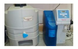
A system designed to produce sterile, filtered ultra-pure water that is free of particles, salts and organic compounds.
