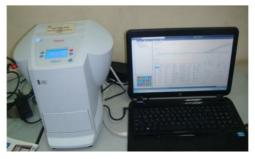
scientific technique of molecular biology based on the polymerase chain reaction which is used to amplify and analysis DNA by detecting the amount of PCR product after each cycle by the incorporation of fluorescent dye into the reaction, the quantification is based on correlation between measured fluorescence intensity and the amount of DNA .
