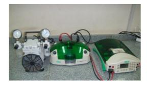
A system for separation of protein according to iso-electric point It offers rapid, simple and effective fraction of protein from complex protein mixture. It offers also two cooling setting:
