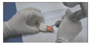
Figure 6. Application of QSR irradiance on bone sample
