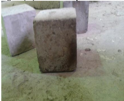
Figure (11) Nano clay specimen at 600 °C
