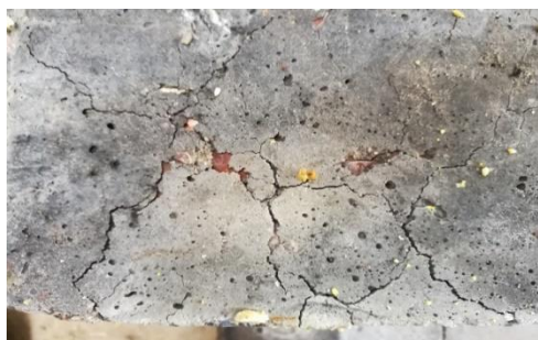
Figure (12) Hybrid mix specimen at 800 °C
