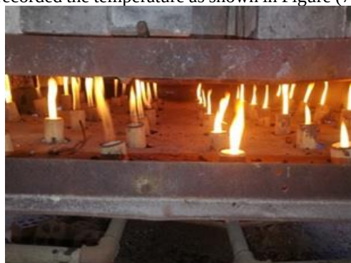
Figure (6) Burning of Concrete specimens
