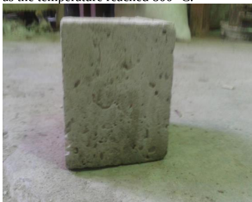
Figure (10) Nano silica specimen at 400 °C
