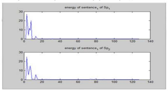
Fig9.Energy distribution of sentence 1 for the two different speakers.
