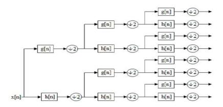
Fig 4.3- levelWavelet Packet decomposition tree.
