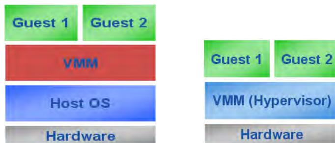
Figure 1.3-A: type II VMM. Figure 1.3-B: type I VMM (Hypervisor)
