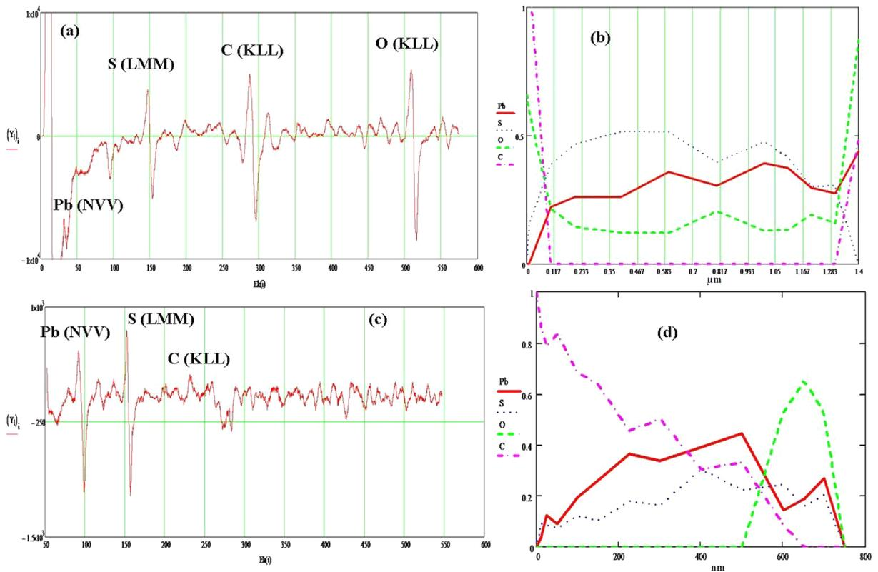
**Fig. 5.** AES spectra of photosensitive PbS films. (a) corresponds to Auger spectrum from samples produced by PVD, (b) shows the ratio of elemental structure to depth of samples prepared by PVD, (c) corresponds to Auger spectrum from samples produced by CVD, and (d) shows the ratio of elemental structure to depth of samples prepared by CVD.
