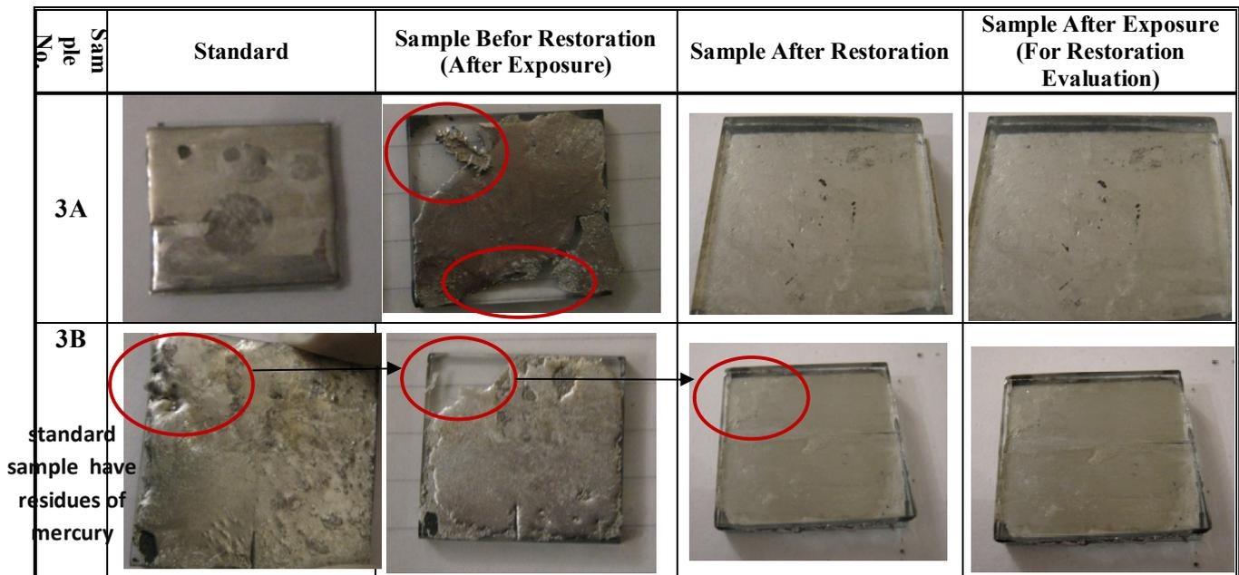
Fig.9. Evaluation of Partial Completion by re-amalgamation process (Photography) visual examination.
