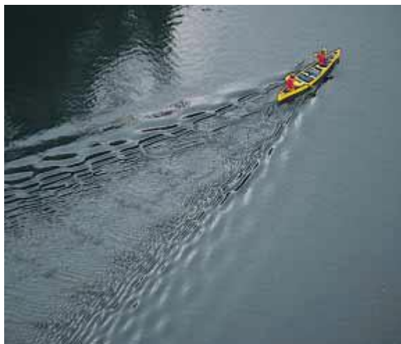
Figure 3.9 The V-shaped bow wave of a boat is formed because the boat speed is greater than the speed of the water waves it generates. A bow wave is analogous to a shock wave formed by an airplane traveling faster than sound.
