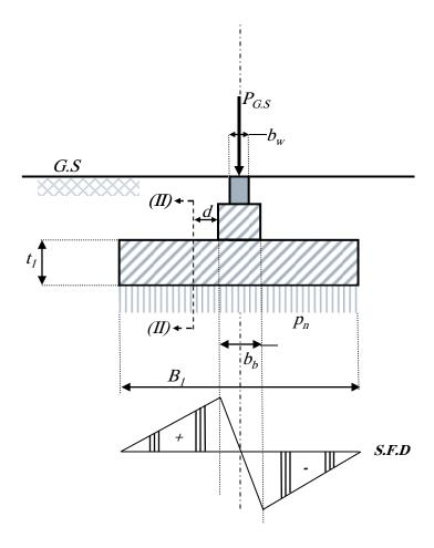
Q<sub>s</sub>: shear force at critical sec. (II).
