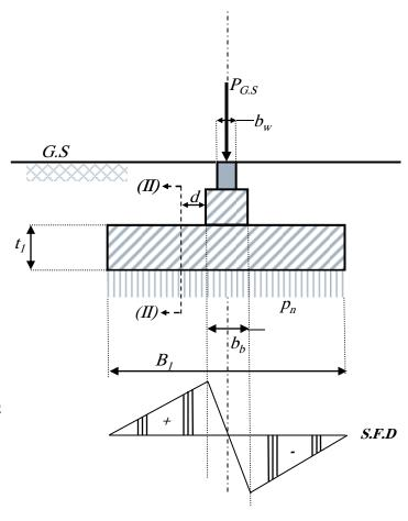
Q<sub>s</sub>: shear force at critical sec. (II).
